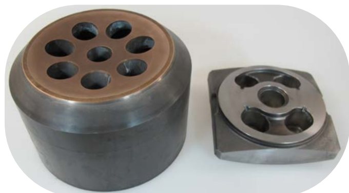
Match lapped 4 15/16" piston pump body and swash plate
